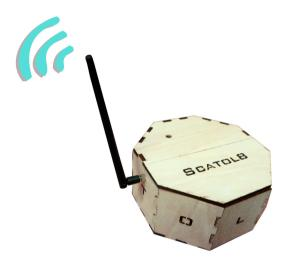
Scatol8<sup>®</sup> is a device that measures environmental variables (energy consumption, air quality, humidity, temperature, ...) and transmits data to a personal computer that stores, processes and displays them through a dashboard, called Crusc8. Thus, Scatol8<sup>®</sup> creates a real-time monitoring system of all variables, that let you assess trends over time, in form of time series analysis. In turn, personal computer sends data
